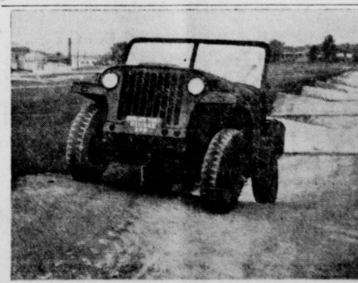
TRY OUT—The Aero Jeep, developed for the Armed Forces, makes a high-speed run over a frame twister course in Aberdeen, Md., to test for strength of springs and chassis. Three feet shorter and 1200 pounds lighter than the standard jeep, this is designed for airborne and other military operations where weight counts.
