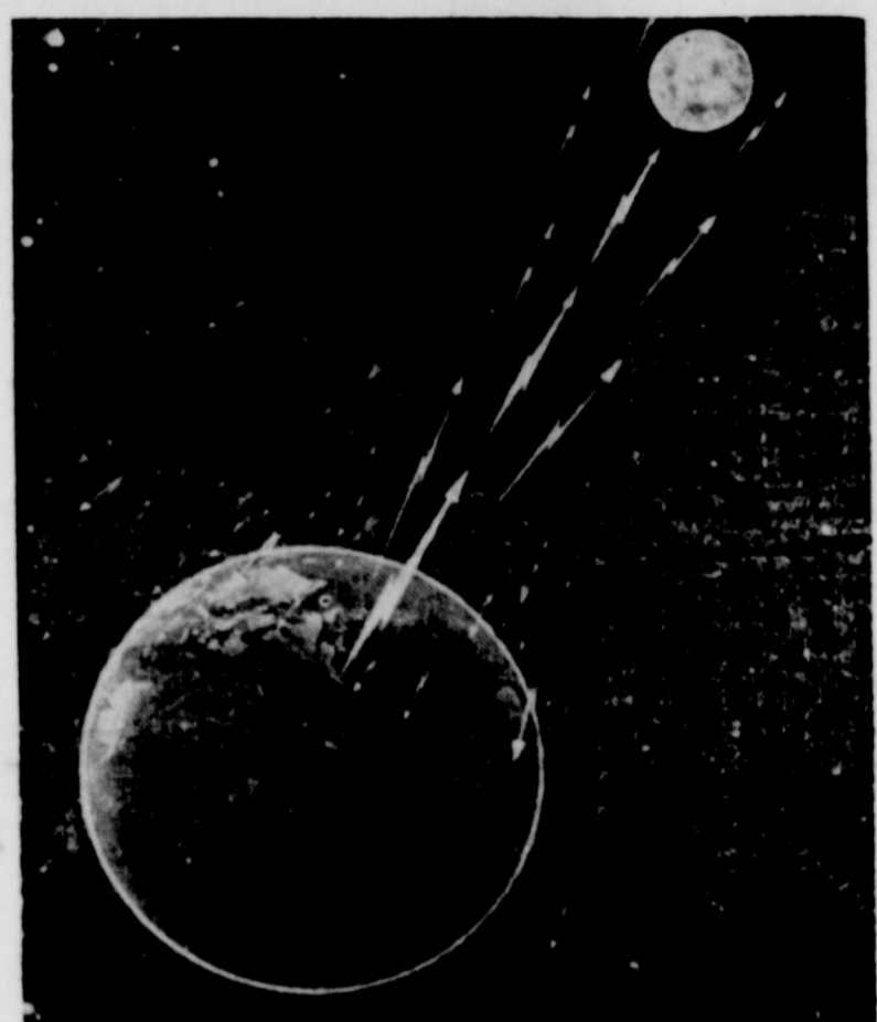
MOON CONTACTED VIA RADAR AGAIN . . . On January 26, the moon was contacted from the earth via radar for the second time. From the Evans signal laboratory at Belmar, N. J., using a radar set specially designed for the purpose, a group of signal corps scientists shot a beam of high frequency energy at the moon and received an answer. The above is a signal corps sketch of the radar contact.
