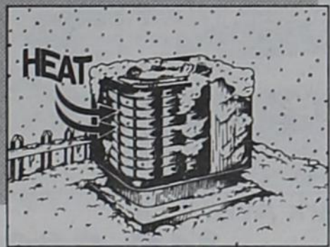
There is heat in the air on the coldest days. The heat pump captures it to warm your home.
