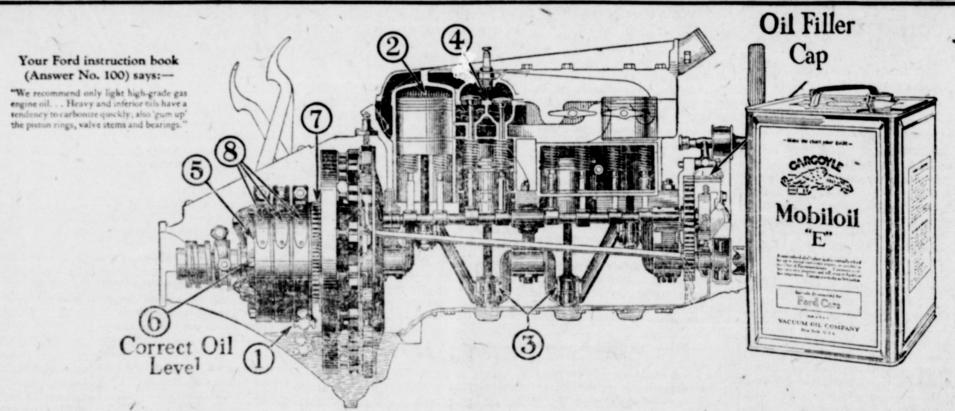
First, you pour in the oil. Your Ford manual tells you to open the top pet-cock on the oil reservoir, and to pour oil into the filler until it runs from this top pet-cock. Suppose you pour in an oil heavier than "E." It is easy to supply too much, unless the oil flows out freely when the upper pet-
