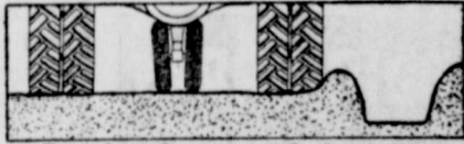
Rear view of tractor with tires set for listing
