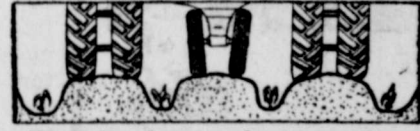
Front view of tractor showing position of tires for first cultivation
