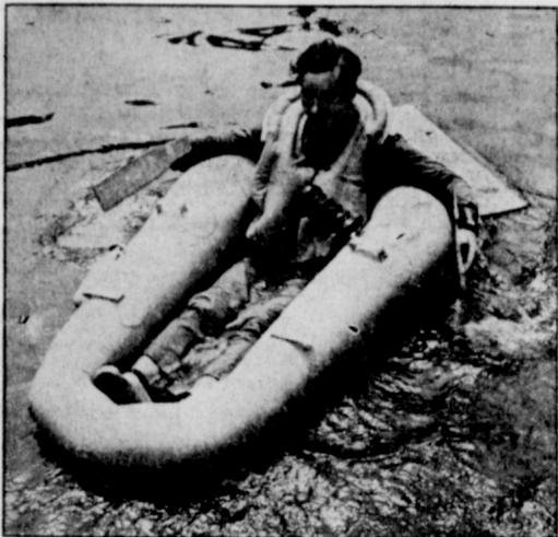
An ingenious new one-man parachute boat for emergency use on single-seater fighter planes is being tested by American armed forces. Ralph Douglas had it inflated in less than 10 seconds in a demonstration of the new life-saver. It's attached to the pilot's seat.
