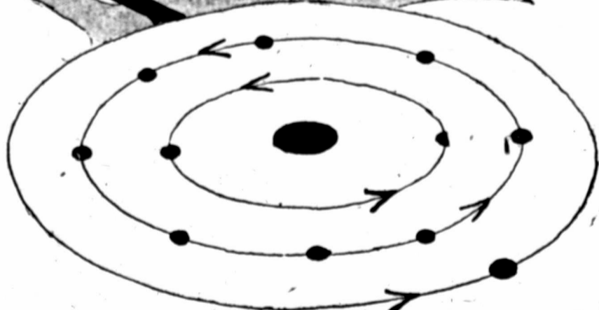
The sodium atom is typical of atomic construction. It has a core of eleven positive units around which revolve in fixed orbits eleven negative units or electrons, thus making up a system very like our solar system. The nature of the element can be changed by knocking one of these units out of the system
