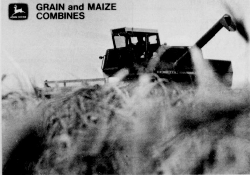
This is the "big boy" of the New Generation Line. Power: 128 observed h.p. Grain tank: 129 bushels. Separator: 55 inches wide. Truly a big combine. A giant in performance. Cutting platforms as wide as 24 feet help it set a new standard for productivity among combines of any make.
