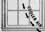
A single pane of glass cools warm air quickly. Cool air drops to floor causing drafts.
