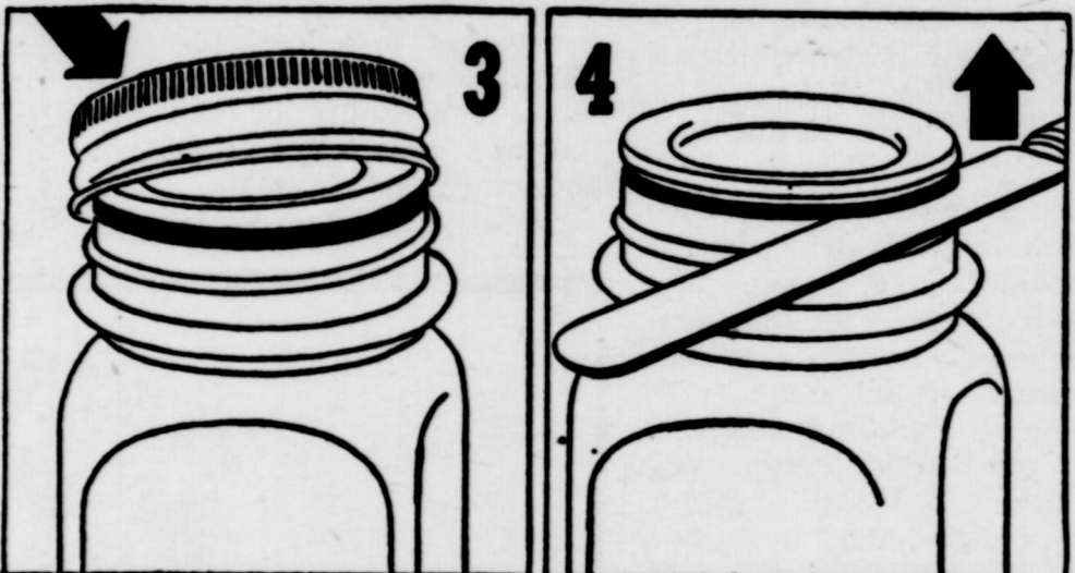
3. Third step: Screw lid and ring down with screw band. Have band fitting loosely during processing. Tighten immediately after processing. When jar is thoroughly cool, screw band may be removed permanently. 4. To open jar before serving contents, release vacuum inside jar by inserting dull table knife under jar rubber.
