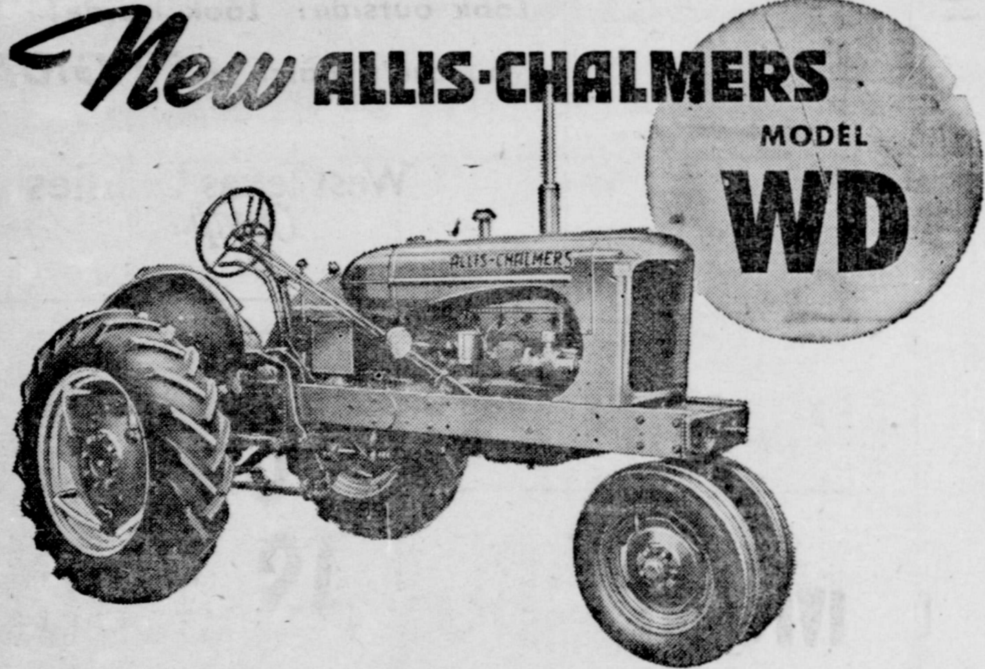
Views of the Allis-Chalmers WD tractor with a 42 gal. Butane tank.
