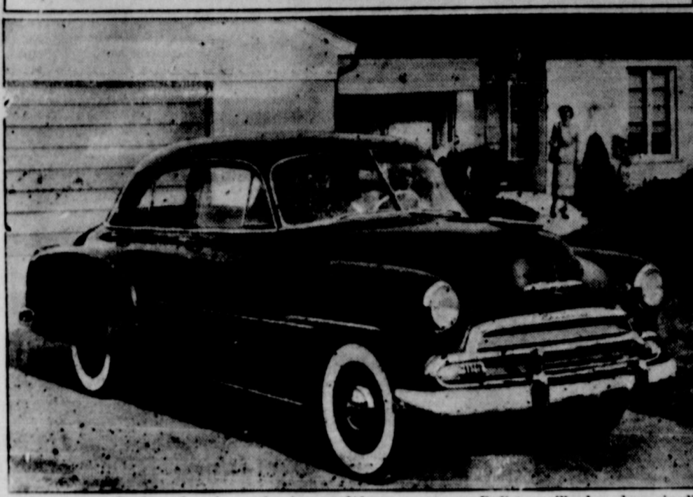
The Styline De Luxe four-door sedan is one of 14 models introduced by Chevrolet as its passenger car line for 1951. Notice in this picture are the rear fender crumple raised. Models also offer added design improvements which accentuate a longer, lower appearance. Radiator grille has been simplified. The decorative body moulding lowered and rear bumper crumple raised. Models also offer added design improvements which accentuate a longer, lower appearance.
