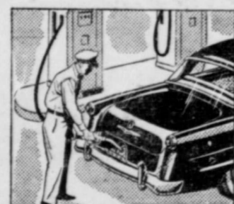
CENTER-FILL FUELING —prevents hose marks, and makes "filling up" easier from either side of gas pump. Shorter gas filler pipe gives you trunk space for an extra suitcase.
