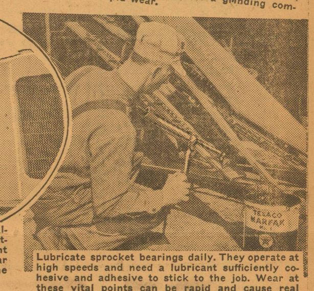
Modern bundle-carriers have fittings for grease-gun lubrication. Bundle-carrier bearings should be lubricated several times daily. Make sure the fittings are cleaned off before you apply the lubrication. If dust is forced into a bearing, it makes a grinding compound, causing rapid wear.
