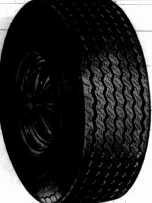
The General Poly-Jet features four-ply construc-
