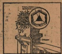
of its depth with tin or zinc, and drained through a one-inch tube to the downspout, or over the edge of the porch. A triangular piece of window screen placed over the drain opening will prevent clogging of the pipe.-Popular Mechanics Magazine.
