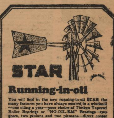
gears, two pinions and two pitmans—direct center lift to pump rod—crosshead, guides and pitmans bearings flooded with oil—a scientifically designed wheel with angle steel arms and braces and ball-bearing turn table. The fans of this new Star are curved to give great efficiency in an 8 to 10 mile an hour wind. Plunger
