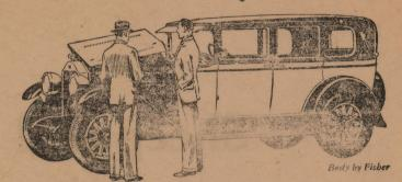
DUICK'S remarkable freedom from vibration is D due primarily to three vitally important factors. First—the inherent smoothness of the Buick Valve-in-Head six-cylinder engine. Secondrubber engine mountings, front and rear. And third—the scientific and almost perfect balance of the entire Buick crankshaft assembly.
