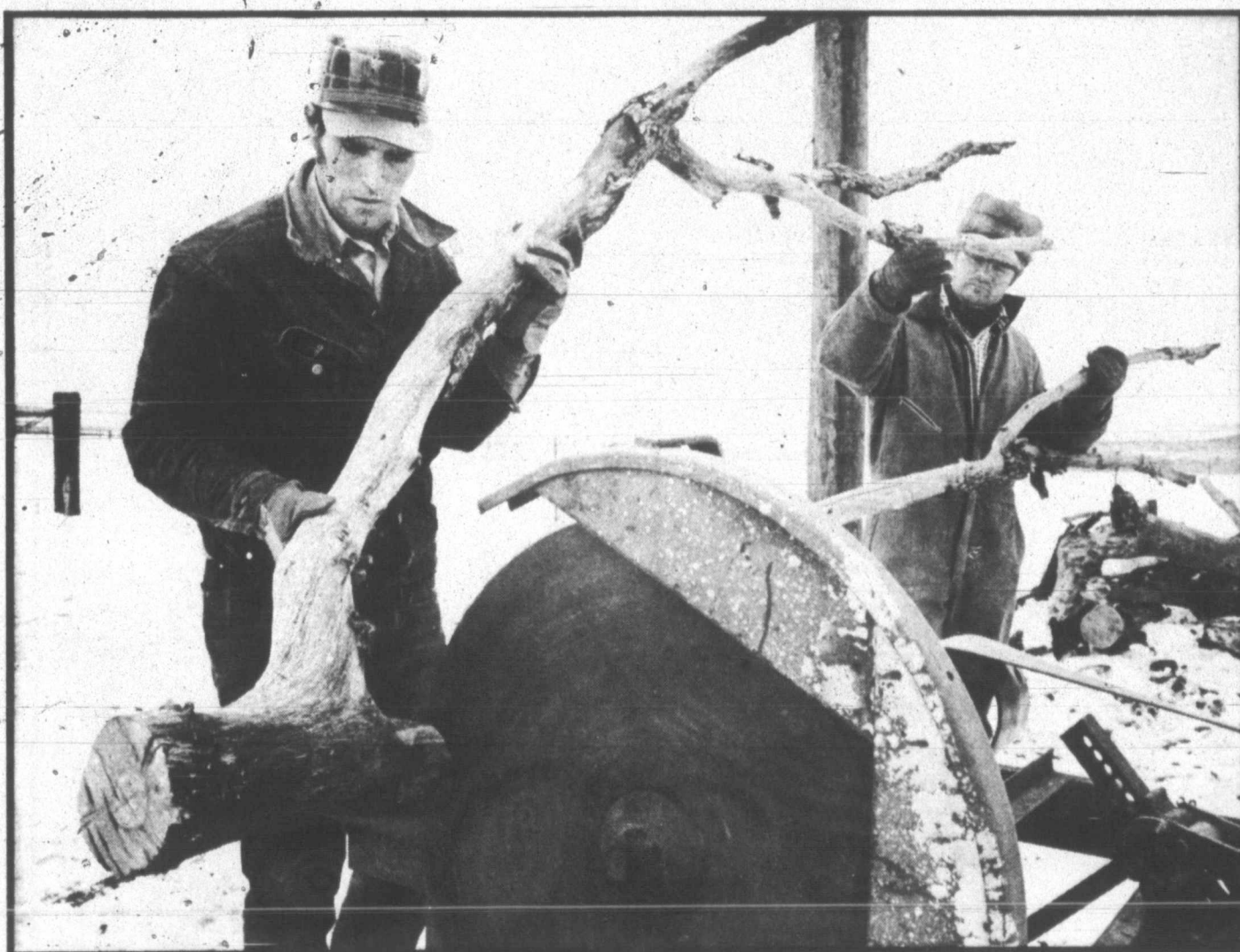
Tom Vick, left, and David Crockett find a belt saw driven by a tractor more reliable than more modern chainsaws.
