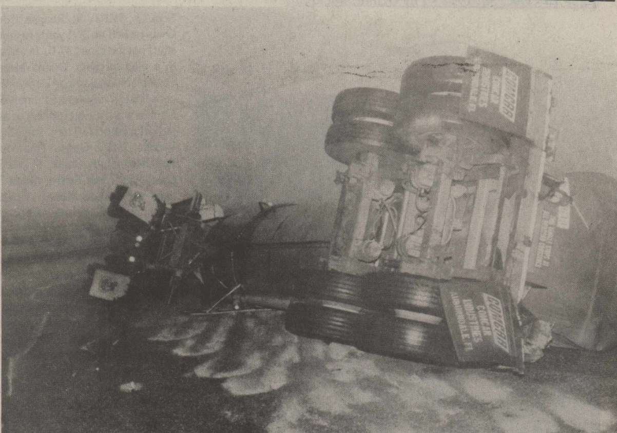
THIS CTL DISTRIBUTION COMPANY TANKER TRUCK of Mulberry, FL overturned on the curve of the service road at the overpass near the truck stop on I-10. Trooper Richard Barton indicated that the truck was carrying a partial load of heavy fertilizer nitrogen solution which shifted on the curve causing the truck to topple over Monday morning. Ozona Stockman photo
