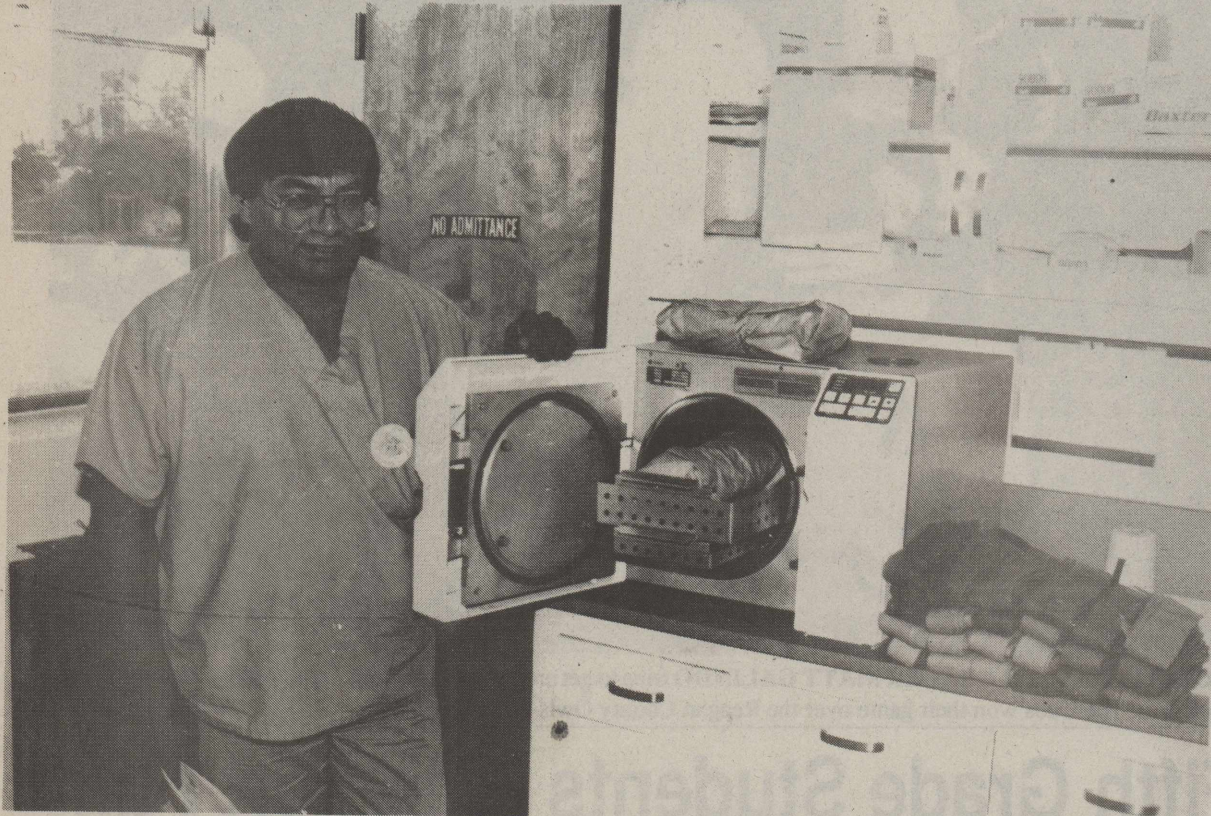
FELIX TRUJILLO is ready to put the hospital's new autoclave to work. The machine, which is used to sterilize surgical instruments, was bought by the hospital with a donation from Crockett County DeerFest Association.
