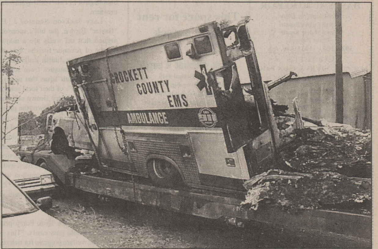
AN ELECTRICAL FIRE in the engine compartment spread throughout EMS II last week, leaving only a charred shell. DigiCam Photo by Scotty Moore
