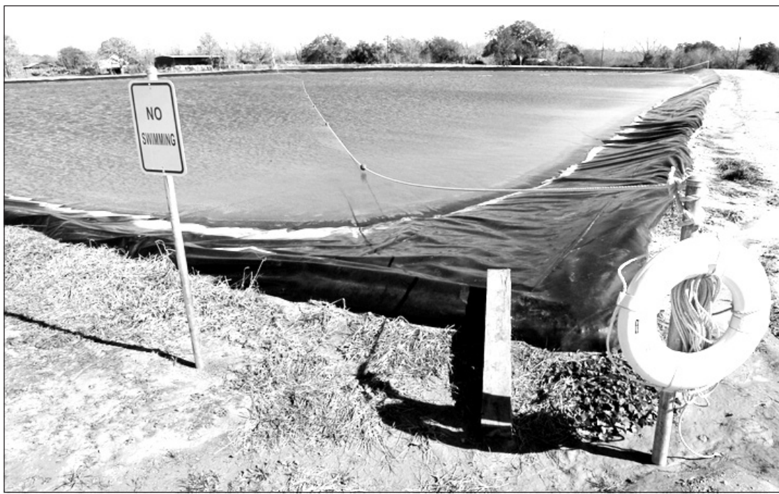
FIELD DISTRIBUTION WATER TANK used in the fracking process of natural gas well drilling in DeWitt County, Texas, complete with life buoy and "No Swimming" sign.
