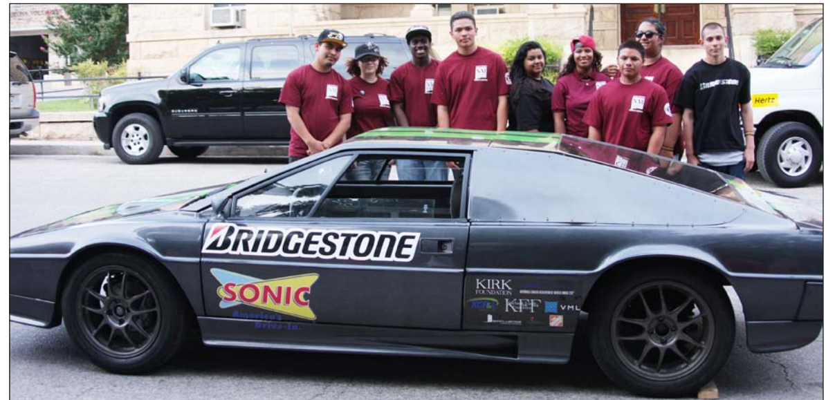
STUDENTS FROM THE MINDDRIVE PROGRAM showed off their electric car "Lotus" during a stop on June 15 at the town square. Lotus has been totally converted into an electric vehicle. Her body has been modified to make her more lightweight and aerodynamic. Lotus is powered by 30 Lithium Ion batteries totaling 96 volts and has a chain-drive motor. The students are driving the car from California to Florida. They also stopped in Fort Stockton, Sonora and Junction over the weekend. MINDDRIVE is an after school program for high school students out of Kansas City, Mo. For more on their journey, visit www.minddrive.org.
