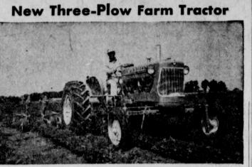
The completely new D-15 farm tractor, featuring three plow and four row capacity, was introduced by Allis-Chalm-ers farm equipment division for the 1961 market at its "Gate-way to the Future" show in French Lick, Indiana. Here the unit is shown with a four-row rear-mounted cultivator work-ing in soybeans.
