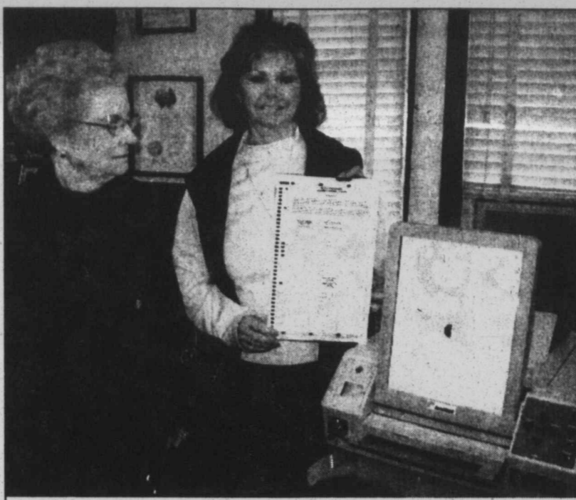
Paper Ballot Printout ... Dovie Miller (left) and Lynn County Clerk Susan Tipton show the paper ballot printed out from the new electronic voting equipment which the county has purchased with grant funding. The ballots may be marked by hand, if desired, or fed into the machine at right to be marked with a touchscreen process. (LCN PHOTO)
