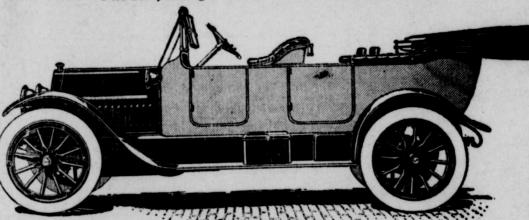
Four cylinders, 4 1-8 inch bore x 5-inch stroke, 116-inch wheel-base. Six passenger body, 34x4 inch Goodrich Tires, Luxurious upholstery Studebaker Jiffy curtains, electric horn, electric lights, electricself starter, clear vision windshield, 3-quarter elliptic springs, Tire holders, detachable, demountable rims,
