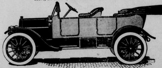
Five Passengers, 4 cylinders, long stroke, 3 1-2 inch bore x 5 in. stroke, 102-in w-base 30 x 3 1-2 Goodrich tires, Demountable Rims, Acetylene gas primer. Stude-baker Jiffy curtains, Electric horns, Prest-o-lite tank, Silk mohair top, Extra rim, ventilating windshield, Speedometer; Tire holder, Tools, elliptic springs
