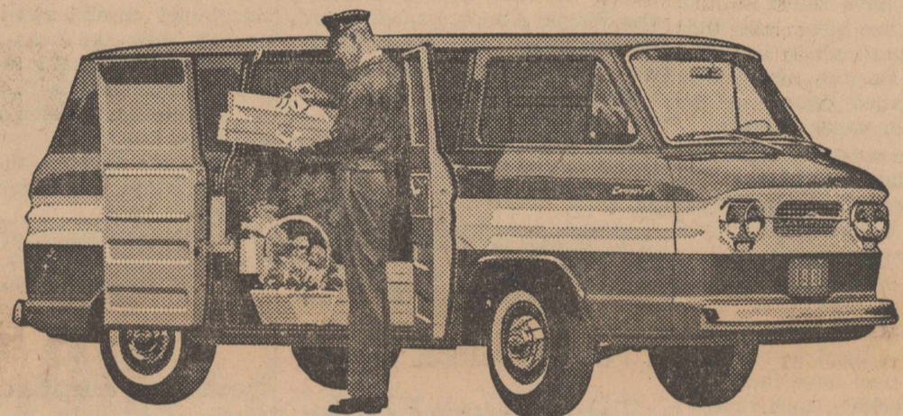
CORVAN—Side doors open a full 49" wide. Loading height is a low 14" lift!
