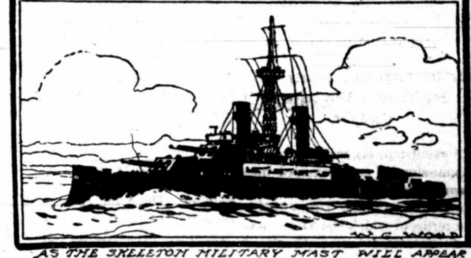
AS THE SKELETON MILITARY MAST, WILL APPEAR ON THE NEW FIGHTING SHIPS
