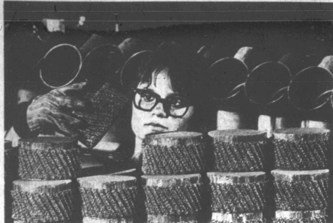
YOU'VE HEARD OF people who get buried in their work. This worker at Tenneco, Inc.'s, Walker Manufacturing Co. appears to be just that. She is preparing the inner elements of catalytic converters for installation in the outer shell at the company's plant in Newark, Ohio.
