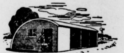
QUONSET 24 —24 feet wide; length variable, in 12-foot sections.
