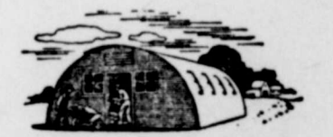
QUONSET 20 —20 feet wide; length variable, in 12-foot sections.
