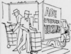
**CRYOGENIC** refrigeration for trucks and other forms of transportation involves use of intense cold (-320 degrees F.) liquid nitrogen. A new system developed by National Cylinder Gas, Chicago, does not inject the nitrogen directly into the cargo compartment but passes it through channels in the wall, floor and ceiling insulation. The compartment is kept nitrogen-free.
