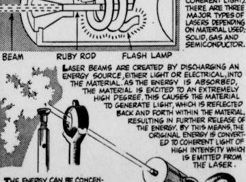
THE ENERGY CAN BE CONCENTRATED TO BLAST A HOLE IN A DIAMOND OR SPOT-WELD METAL, A CONCENTRATED LASER BEAM HAS EVEN BEEN REFLECTED OFF THE SURFACE OF THE MOON.
