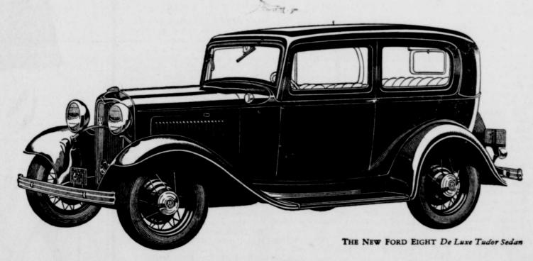
Eight-cylinder, 90-degree V-type, 65-horse-power Engine \* Vibrationless Roomy, Beautiful Bodies \* Low Center of Gravity \* Silent Second Gear Synchronized Silent Gear Shift \* Seventy-five Miles per Hour \* Comfortable Riding Springs \* Rapid Acceleration \* Low Gasoline Consumption \* Reliability
