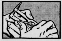
Crank is now used to turn shaft. Oil film ruptures and bearings "seize." Shaft extremely hard to turn. You can even bear the metal-to-metal con-
