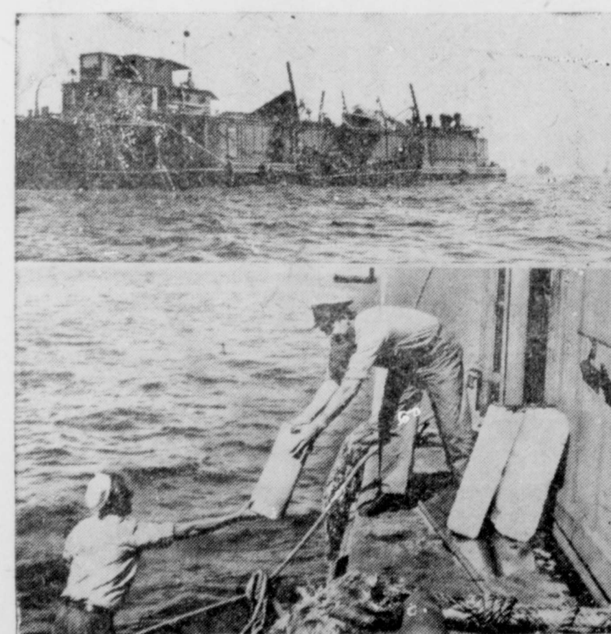
This may look just like an ugly barge to you, but it is the corner drugstore to thousands of men of the Pacific fleet. The barge has a plant that can turn out ten quarts of ice cream every seven minutes. It can also produce five tons of ice daily. Below: A chief storekeeper is handing out a container of ice cream to a "customer" who came for it in a small boat.
