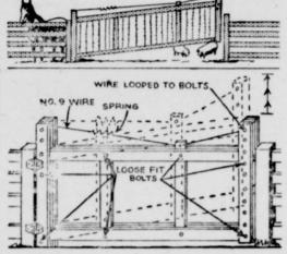
When this unusual stock gate is unlatched, the end automatically will rise several inches off the ground enabling it to clear rocks, snow and other obstacles. If provided with two latches, one mounted a distance above the other, the gate may be left closed and in the raised position to provide a creep for smaller animals while still confining the larger ones. It is constructed and strung with barbed wire.
