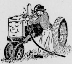
Wash your tractor thoroughly. Dirt breeds rust and hides cracks, tire breaks and bolts that need nuts.
