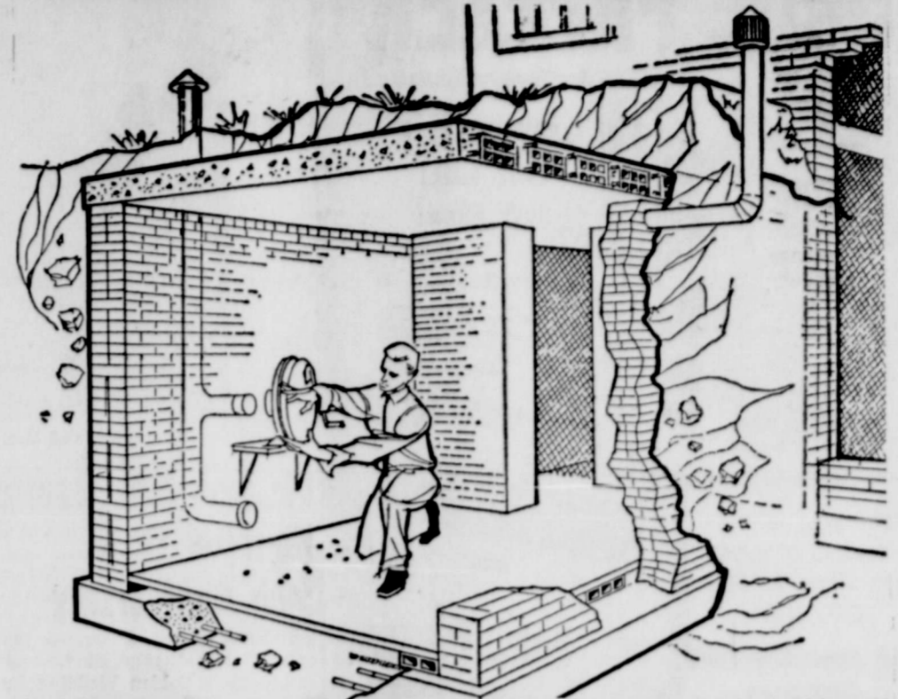
DUAL-PURPOSE underground fallout shelter of clay masonry construction and designed to be built as part of new house would combine some nuclear blast protection, excellent shielding from fallout, and the usefulness of an ordinary basement room. This six-person shelter, which would cost about $650 including $250 to $300 for labor, is one of eight designs in the Defense Department's new "Family Shelter Designs" handbook available at state and local civil defense offices.
