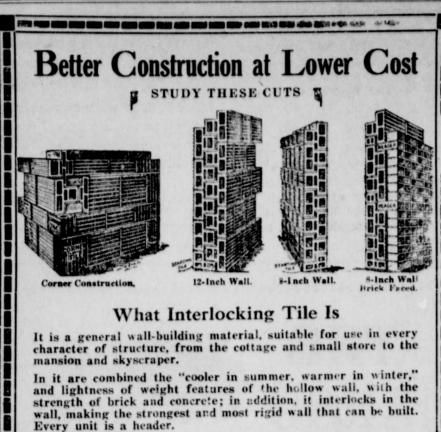
Interlocking Tile is not to be confused with ordinary square tile, which is only designed and intended for partition, and other interior non-load-bearing walls.
