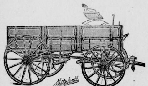
The axles are of split hickory, bolsters, sand boards, reaches and hubs of oak, spokes of hickory, the boxes of yellow poplar. Paint is never used to cover up cheap materials. You can look right on the under side of the gear and see for yourself how good the timber is.
