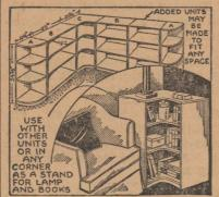
All of the units in the sketch are well proportioned with deep shelves and are especially designed to be made by the man who is handy with hammer and saw. Patterns are available with actual-size cutting guides for the curved shelves. Stock widths of lumber are used and the pattern lists all materials needed. Only the simplest hand tools are required.
