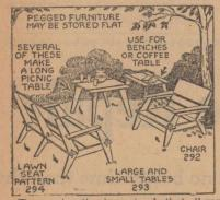
The construction is so simple that all you eed is stock widths of lumber, a hand aw, a screw driver and a brace and bit the holes for the pegs.
