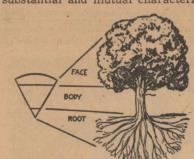
Face, body and root are important in electric welding. Drawingcourtesy Lincoln Electric Co.
