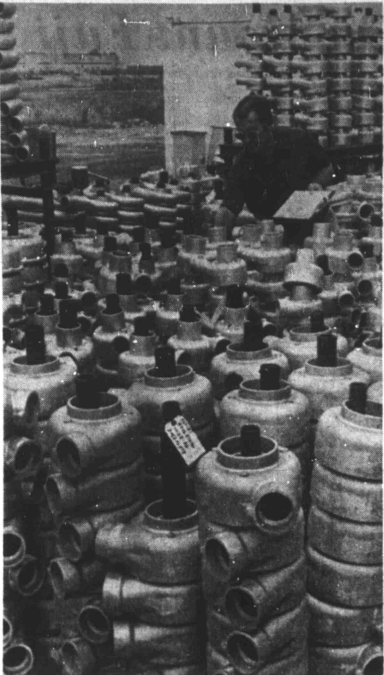
HOUSING INSPECTOR — Jack Mitchell keeps tabs on turbocharger compressors at Garrett Corporation in Torrance, Calif. The turbochargers are designed to boost the power output of engines on tractors, trucks, off-highway vehicles and cars. (AP Laser-photo)
