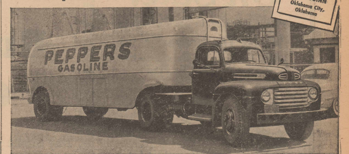
Ford Model F-8 BIG JOB shown has a Gross Vehicle Weight rating of 21,500 lbs.; Gross Combination Weight rating as a tractor is 39,000 lbs.
