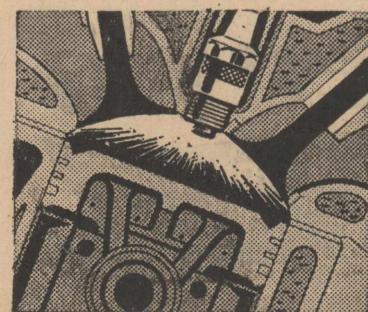
Hemispherical Combustion Chambers the engineering reason why no other American passenger car engine today can match FirePower performance.
