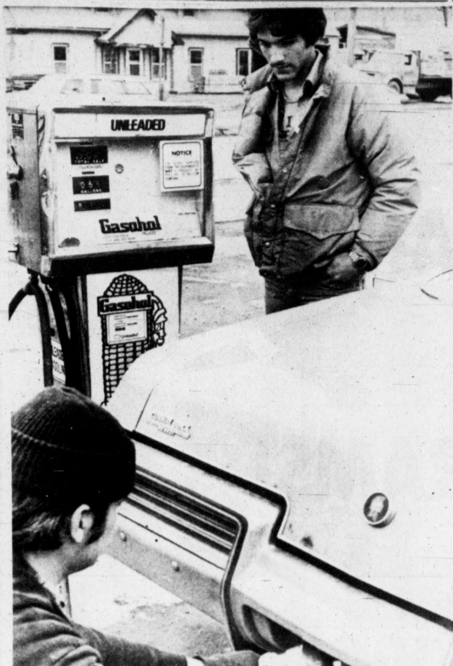
Des Moines, Iowa, service station attendant Bob Lenihan, left, fills Dave Stefanic's fuel tank with gasohol. Gasohol, a blend of 10 percent grain alcohol and 90 percent unleaded gas, has a higher octane rating than unleaded gas and is competitive in price to premium. The blended fuel is sold in more than 400 stations in Iowa. (AP Laserphoto)
