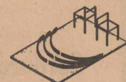
You simply make an erection scaffold slightly shorter than the height of the size building ordered. Lap and bolt half arches on the ground as indicated.
