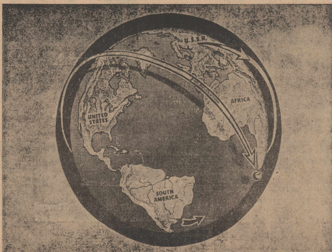
RUSS SATELLITE . . . Artist's conception of orbit (white arrow) of Soviet man-made 23 inch moon circling earth every hour and 35 minutes at height of 560 miles and speed of 18,000 mph. Black arrow indicates rotation of earth from west to east.
